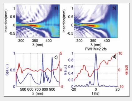
Single-cycle hollow-core fiber (HCF) compressor: Measured (a) and retrieved (b) SHG D-scan traces. (c) Measured spectrum (blue) and retrieved spectral phase (red). (d) Reconstructed temporal profile for a post-compressed pulse in an Ar-filled HCF (P=409 mbar) with PC1332 spectral phase compensation, corresponding to 2.2 fs (1.04 cycles at 760 nm). Figure adapted from [2].
