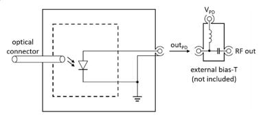
Block diagram of FP1015a. An external bias-T of ≥ 30 GHz (-3-dB) is required.
